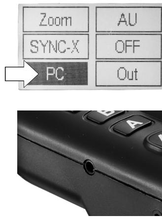
**IMPORTANT!** It is not possible to change the power of the light connected with the synchronization cable. The cable is not included in the set. A second transmitter is required for this function.
