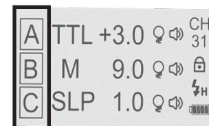
**IMPORTANT!** To get other lights in Slave mode to receive the signal, they must operate on the same channel as the transmitter.
