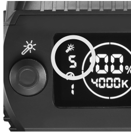
2. Light effect activation indicator will appear on the LCD together with the number of the selected effect (see table below)
