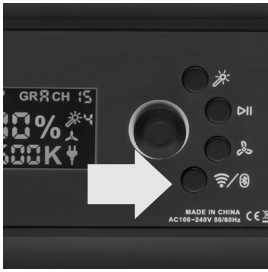
(1) Press the wireless control mode button until the channel indicator on the LCD starts to blink.
