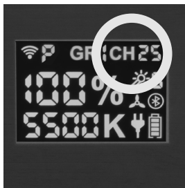
(2) Turn the control dial to set channel.
